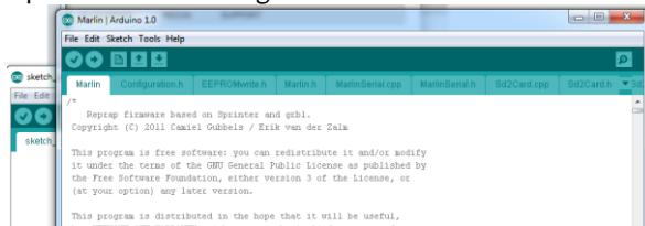
A new window will pop-up, with all the source firmware files. All the settings for the FelixPrinter to work correctly are configured. Feel free to browse around the files to get a better understanding of how it all works.
