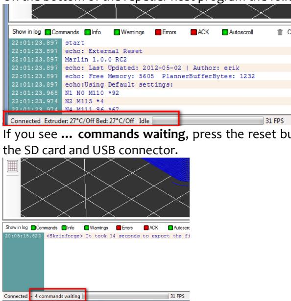
If you see ... **commands waiting**, press the reset button on the side of the electronics board. Next to the SD card and USB connector.
