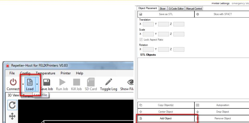
Press the *Load* button or in the Object placement tab, *Add Object* button.
